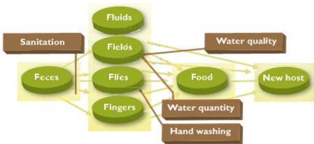
Figure 1: Transmission routes of diseases by feces and its barriers or prevention methods
